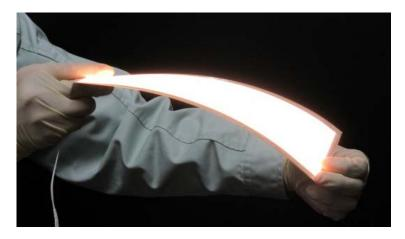
This flexible OLED is based on "P11 series" (Lamp color) and its size is 284mm x 71mm. This panel achieved both the flexibility and the brightness equivalent to P11 (front brightness 5,000cd/m2).
